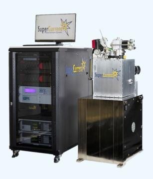
The HTS-110 8 T Electrical Transport Measuring System provides automated measurement of electrical transport properties as a function of magnetic field, field angle and temperature. Completely cryogen-free Ic  $(T,B,\theta)$  to over 800 A, with sample cooling to T<20 K.
