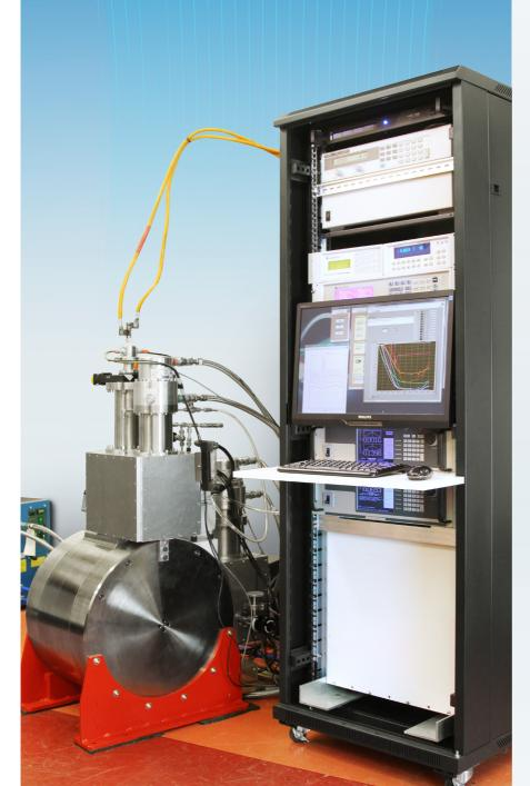
The HTS-110 8 T Electrical Transport Measuring System provides automated measurement of electrical transport properties as a function of magnetic field, field angle and temperature. Completely cryogen-free  $I_c(T,B,\theta)$  to over 800 A, with sample cooling to T<20 K.
